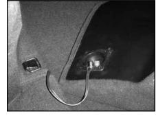
**STEP 8** Attach the speaker wire to the terminal on the Stealthbox<sup>®</sup>.
